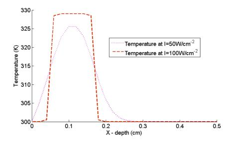
Figure 5: Variation of the Temperature under Depth of Tumor on the Different Values of Intensity of Laser Light
