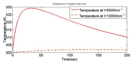
Figure 6: Variation of the Temperature with Timeon the Different Values of Intensity of Laser Light CONCLUSIONS
