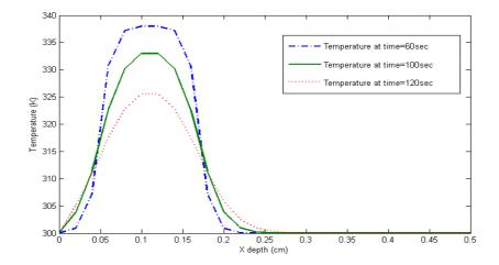
Figure 2: Variation of the Temperature under Depth of Tumor with Different Times
